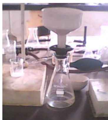
Fig 4: Vacuum Filtration Apparatus
